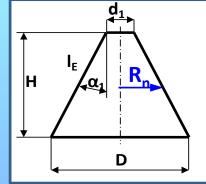
Check of the shell against a stability loss between two reinforcements (it is cylindrical parts = shell and neck). (the cone is without any reinforcement  $\rightarrow$  L = H)
