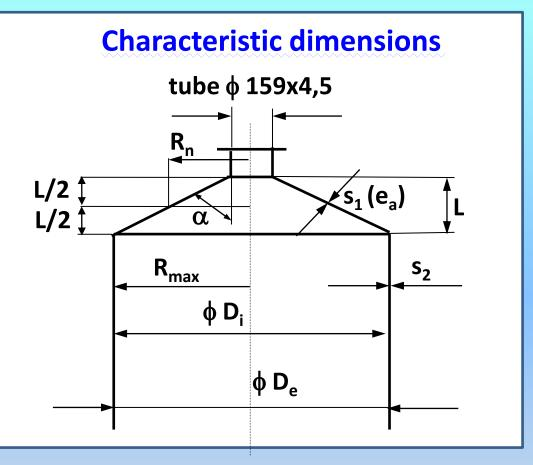
Internal radius of cylindrical shell  $R_{max} = D_i / 2 = 1486 / 2 = 743 \text{ mm}$  (as in the case of ES for cylinder is not the analyzed thickness calculated, but is estimated )
