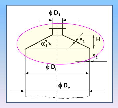
Sketch of cylindrical vessel with conical cover and neck
