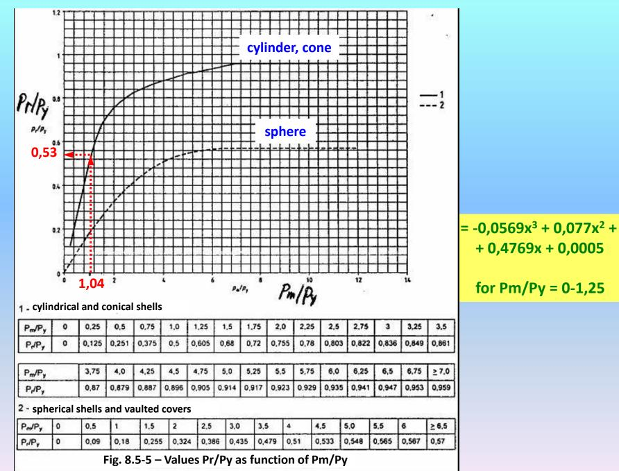
Maximal calculating overpressure for the realized wall thickness must conform to the condition (8.6.3-5)
